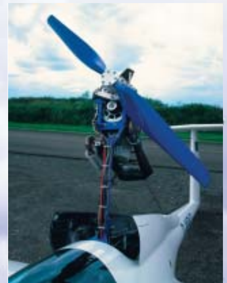
The heart of the Apis ® 2 powerplant is an air-cooled single cylinder Hirth F 33 B
